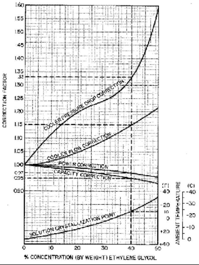
**Example:** Determine concentration of inhibited ethylene glycol to protect the system to  $-23^{\circ}\text{C}$  ambient temperature at zero flow.
