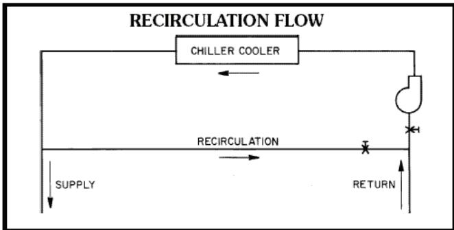
**Maximum cooler flow** — The maximum cooler flow (> 5 gpm/ton or < 5° F rise [> 0.09 L/s · kW or < 2.7° C rise]) results in practical maximum pressure drop through cooler.
