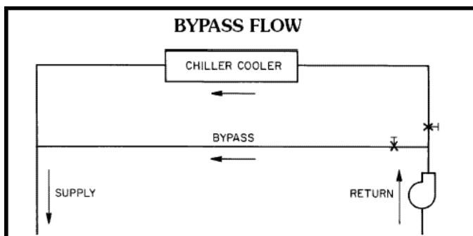
**Variable cooler flow rates** — Variable rates may be applied to standard chiller. Unit will, however, attempt to maintain a constant leaving chilled fluid temperature. In such cases, minimum flow must be in excess of minimum flow given in Minimum Cooler Fluid Flow Rates and Minimum Loop Volume table, and flow rate must change in steps of less than 10% per minute. Apply 6 gal. per ton (6.5 L per kW) water loop volume minimum if flow rate changes more rapidly.
