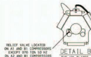
RELIEF VALVES ARE EQUIPPED WITH A 3/8" SAE FLARE FOR FIELD CONNECTION
